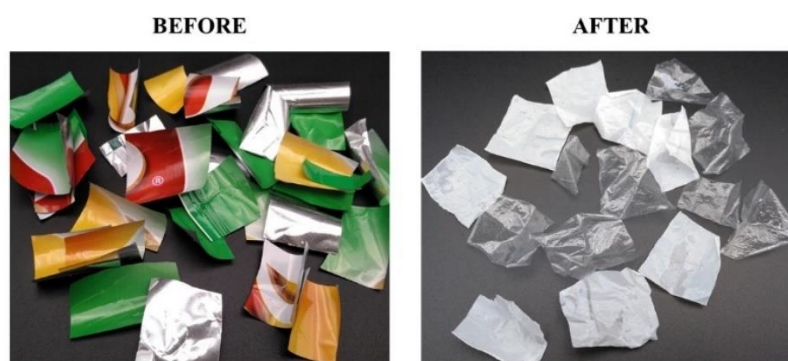
Figure 8: Delamination of multilayer plastic film 150
